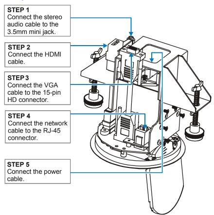
Figure 3: Connecting the Cables (from below)
